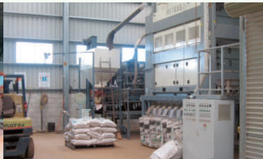
NQTS has commissioned a new state of the art seed grading plant which will increase productivity and fine tune the cleaning of all seeds. The Petkus M 15 3.6 is the latest machine in the range, imported from Germany. NQTS can now grade, size and process legumes, grasses and grains with the greatest of ease.
