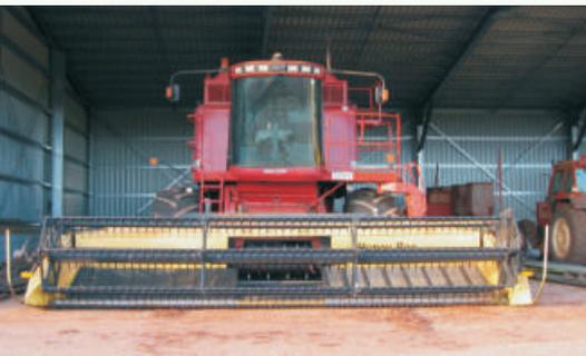
When harvesting legumes care must be taken not to damage seed. NQTS uses a CASE 2388 Rotary Harvester to ensure that the seed is not split or knocked around during harvesting.
